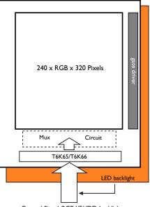
Control Signal, RGB I/F, VDD, backlight
